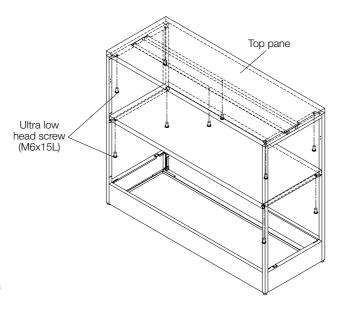
\* Hold together firmly to ensure that there are no gaps between the side frame and the shelf.
